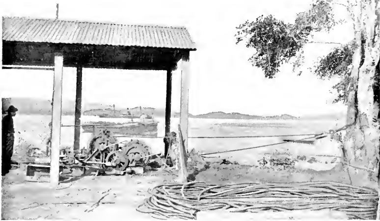
LOADING THE "EARNWELL" FROM LIGHTERS HAULED BY A STATIONARY ENGINE ON SHORE.
